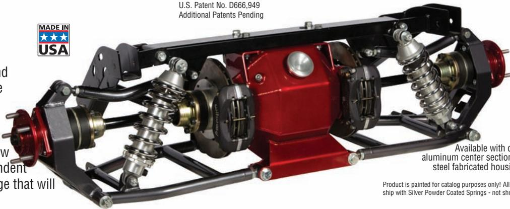
Available with cast aluminum center section or steel fabricated housing.
