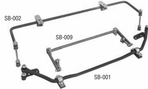
\*SB-001 fits '33-'34 Ford with relocation of mounting holes in frame.
